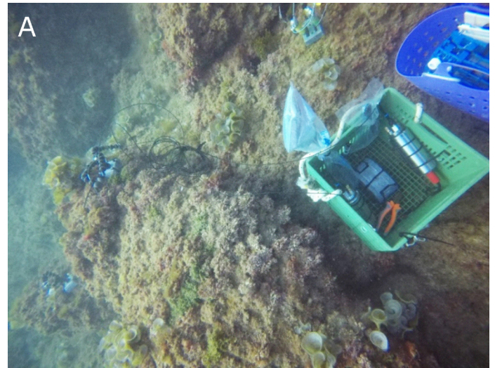
Figure 1A. The underwater set-up of the AquapHOx-Logger. The instruments were very easy to carry and deploy. We secured the AquapHOx-LX in a milk crate for protection
