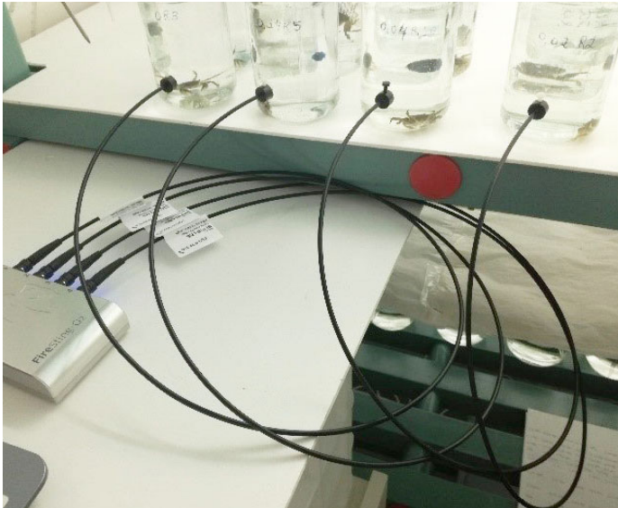
Fig. 1 4 channel oxygen meter FireSting oxygen meter connected to a PC, with optical fibres connected via adapters to experimental chambers (sealed glass container with crab) for contactless read-out of integrated oxygen sensor spots
