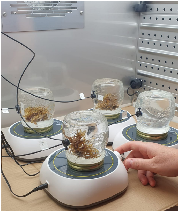
Fig. 1 Light set-up for oxygen production measurements. One jar is filled only with filtered seawater and used as a control
