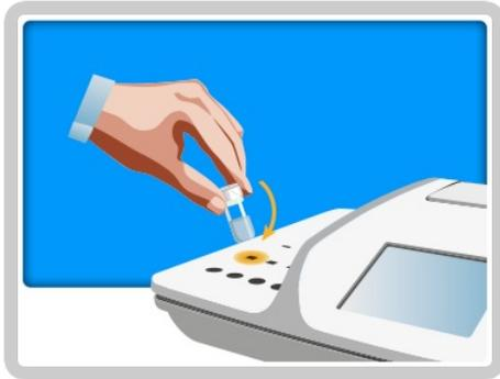
**14.** Place the cuvette in one of the incubation cells and start the timer by pressing the timer icon.
