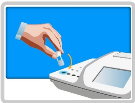
**10.** Select the cuvette to be read from the display. Place the cuvette in the cell marked with the blue light and press READ.
