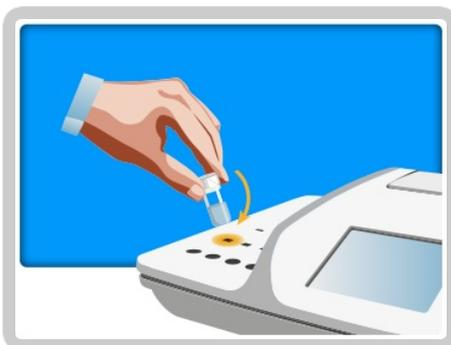
**2.** Place the test tubes containing reagent R1 in one of the incubation cells and let them warm for at least 5 minutes. Place an extra test tube if blank reactive reading is required.
