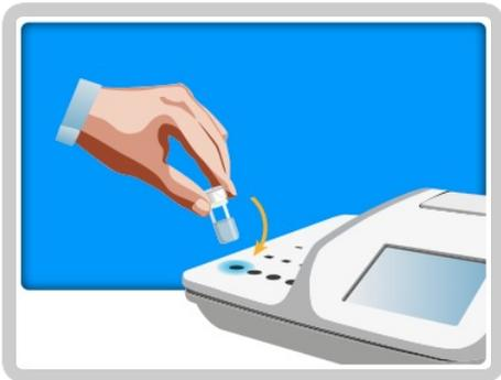
**16.** Place the cuvette in the cell marked with the blue light and press READ to perform the photometric reading.
