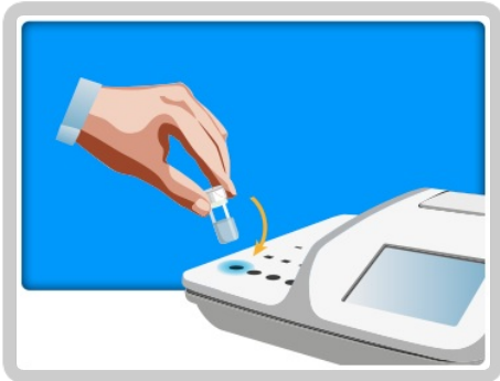
13. Place the cuvette in the cell marked with the blue light and press READ to perform the photometric reading.
