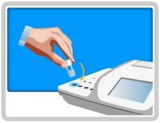
**11.** Select the cuvette to be read from the display. Place the cuvette in the cell marked with the blue light and press READ.
