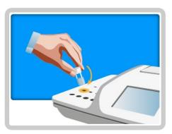
**7.** Place the cuvette in one of the incubation cells and start the timer by pressing the timer icon.
