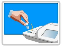
**14.** Place the cuvette in the cell marked with the blue light and press READ to perform the photometric reading.
