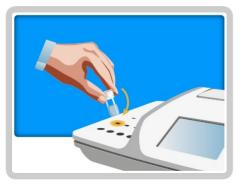
**10.** Place the cuvette in one of the incubation cells and start the timer by pressing the timer icon.
