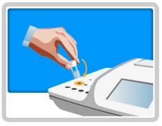
**18.** Place the cuvette in one of the incubation cells and start the timer by pressing the timer icon.
