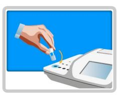
**19.** Place the cuvette in the cell marked with the blue light and press READ to perform the photometric reading.
