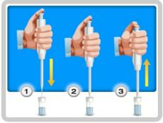
**8.** Place the sample in the cuvette. Keeping the tip immersed in reagent, press and release the piston of the pipette several times.
