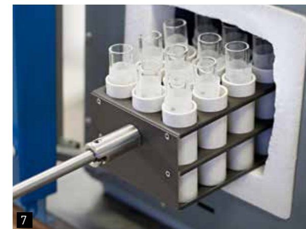
The incinerating module with a long handle makes handling of samples easier.
