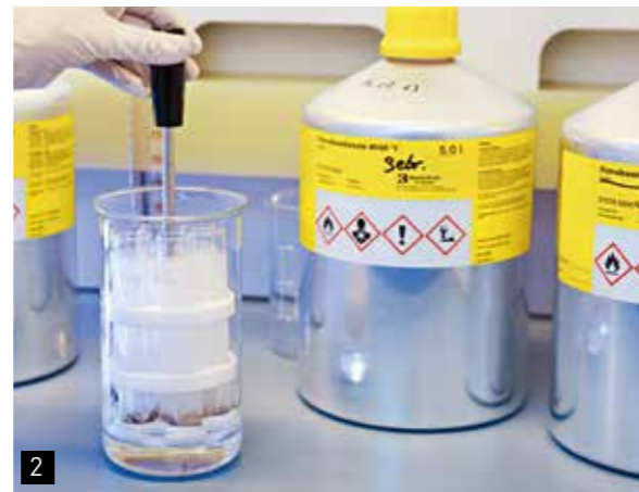
Convenient, time-saving degreasing with solvents in the degreasing module. 6 samples can be treated at the same time.
