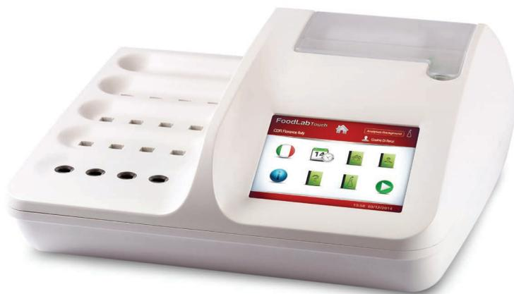
It works using a colorimetric reading at 630 nm that determines the proportional concentration of acid in the sample. Free fatty acids in the sample, at a pH value less than 7.0, react with a chromogenous compound and decrease its colour. The decreasing of the colour expresses the percentage of acid. The kind of acid depends on the kind of matrix. The most common used biofuels are low quality palm oil, rapeseed oil, sunflower oil, soybean oil, frying oil or waste oil.
